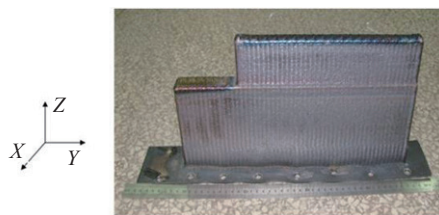
图1 激光直接沉积成形A-100钢试样 Fig.1 Laser deposition shaping A-100 steel
